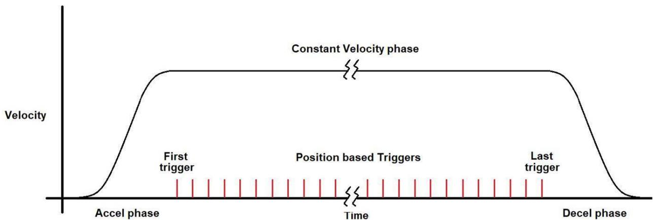
Figure 1: Typical Move Profile with Triggering
