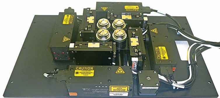
Figure 1: Capable of capturing and processing 350 million pixels per second, a multicamera system features four 20X, 0.80-NA objectives on a 36-mm pitch.
