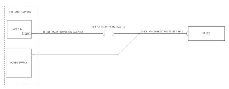
Next, connect the RS-232 breakout adapter (65-5741) to the main stage cable. Connect the Moxa adapter to the adapter cable end(s). The main cable should then be connected to the stage, and the power supply. The system can be powered on, and a connection attempted from the host machine. For more information on the pinout, I/O, connections and cabling, see the SmartStage User Guide.
